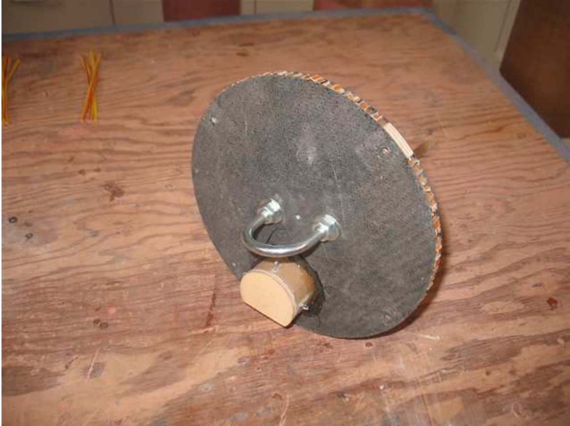
After cutting and fussing here is the nose cone bulkhead ready for mounting into the nose cone shoulder. Note the cotter pins holding the cap in place.
