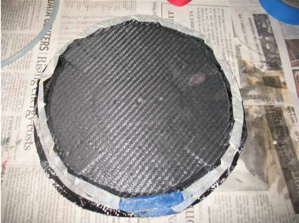
Here is the bulkhead after removing from the vacuum bag. It is ready for final shaping and drilling.
