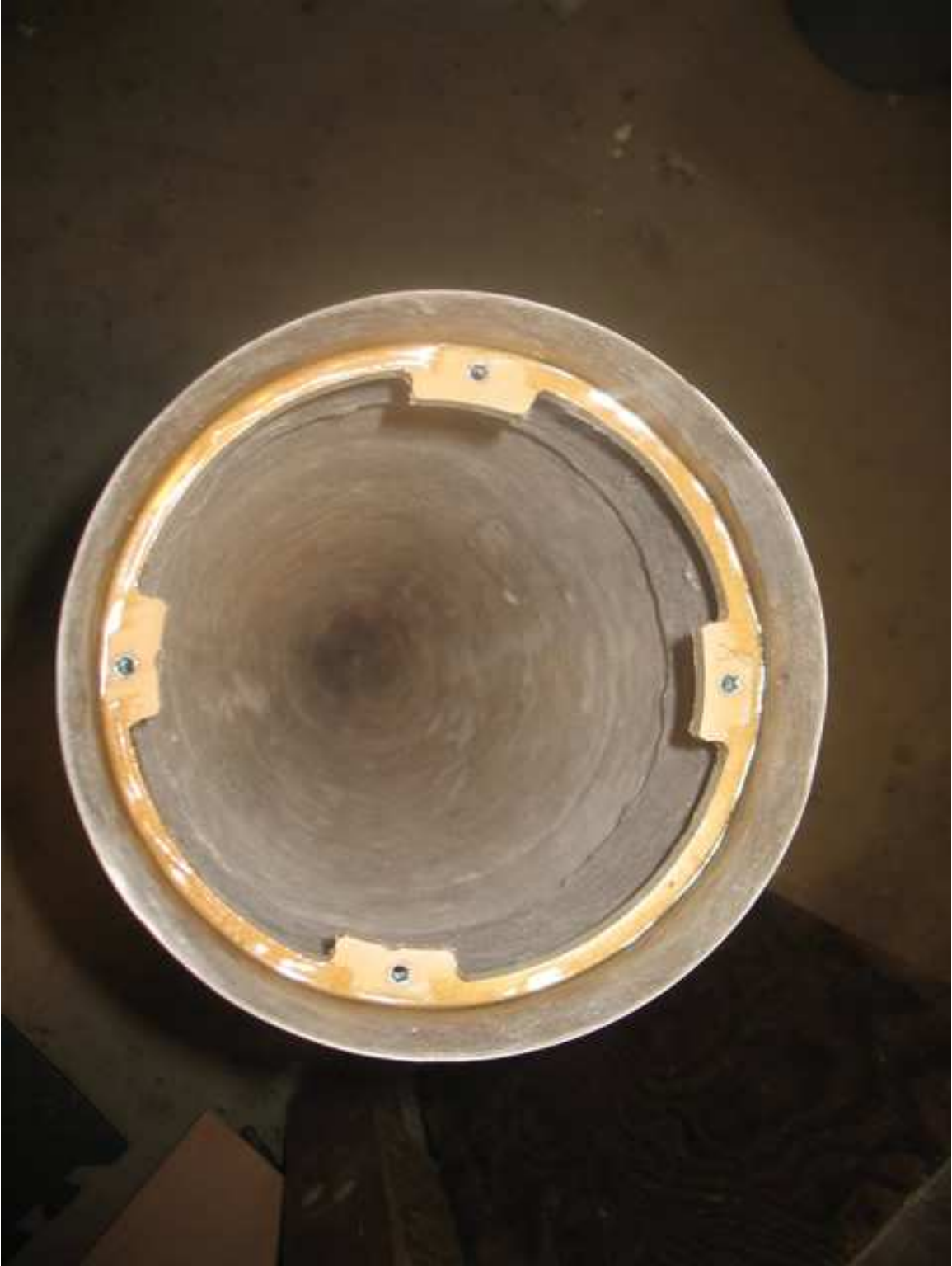
I made a 3/8" plywood shoulder with T-Nuts for mounting. This is glued into the nose cone shoulder.
