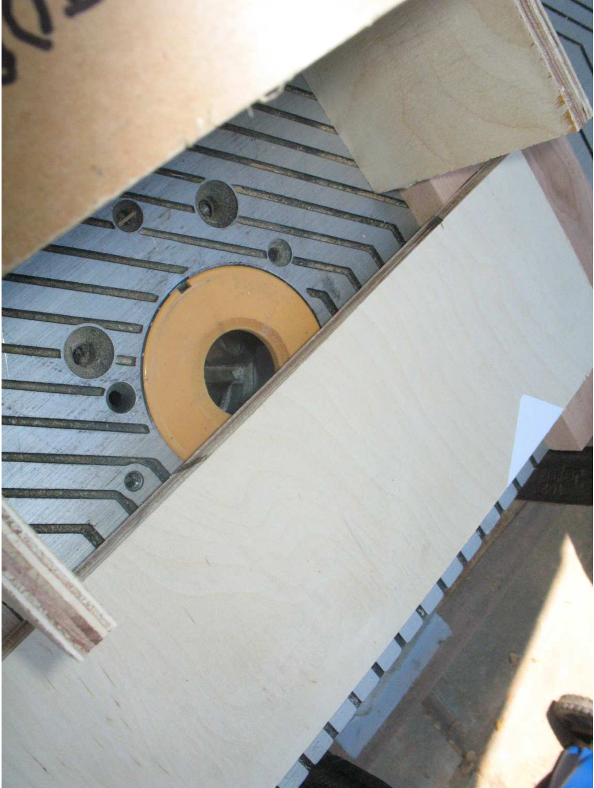
This is clamped at the right location for a 5/16 wide cut.
