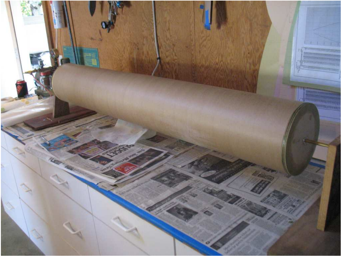
The reinforcing disks and end caps are installed and tightened. This is mounted on a couple of stands to get the airframe up off the workbench so it can be rotated easily.
