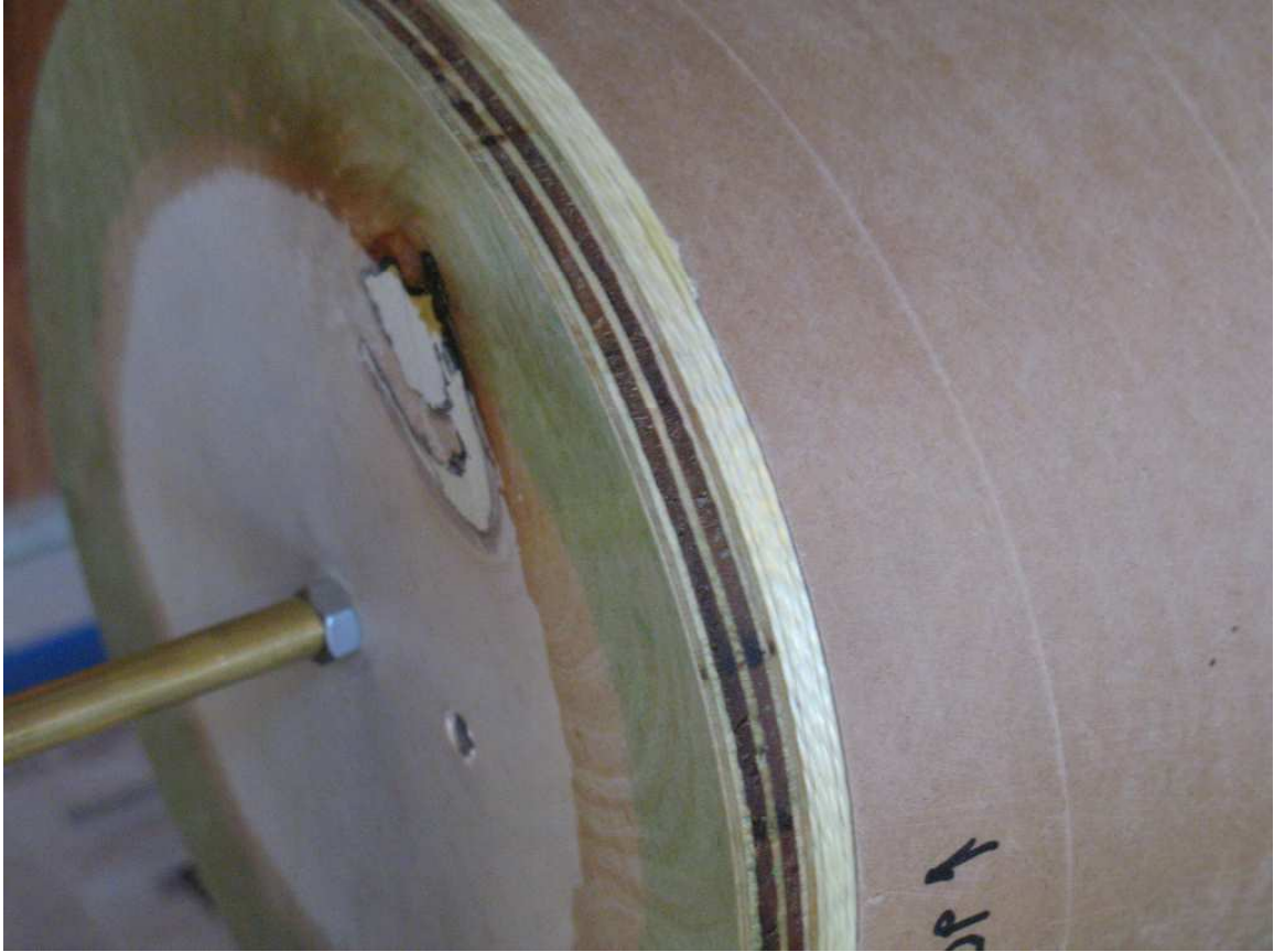
Once the shoulder is filled up the end is again tacked with CA.
