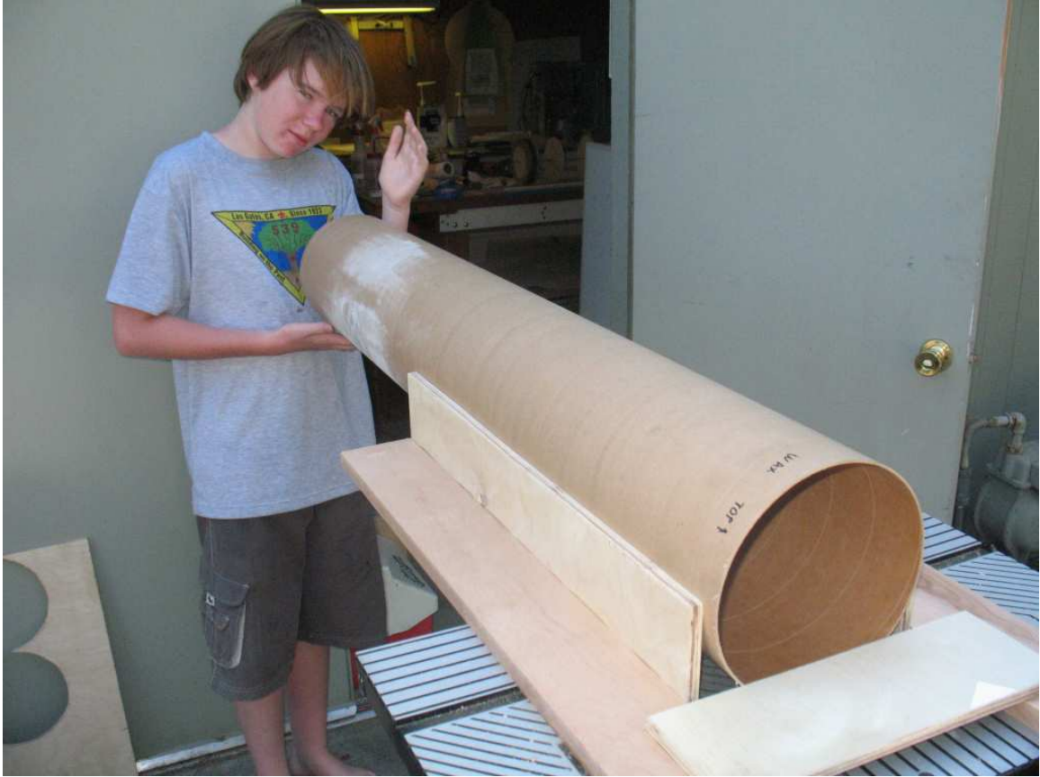
Now the airframe is placed in the cradle and the router turned on. Phil stabilizes the aft end.
