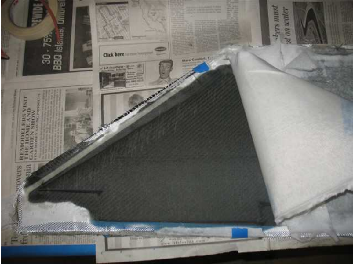
After baking for 8 hrs and while it's still green (not sticky but not fully cured) I peel off the peel ply – beautiful!
