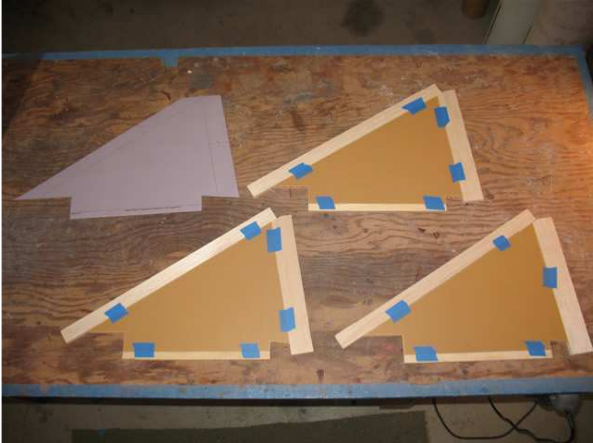
I stripped 1" and 1.5" balsa and taped them to the core. I also added the air-ply for the root.
