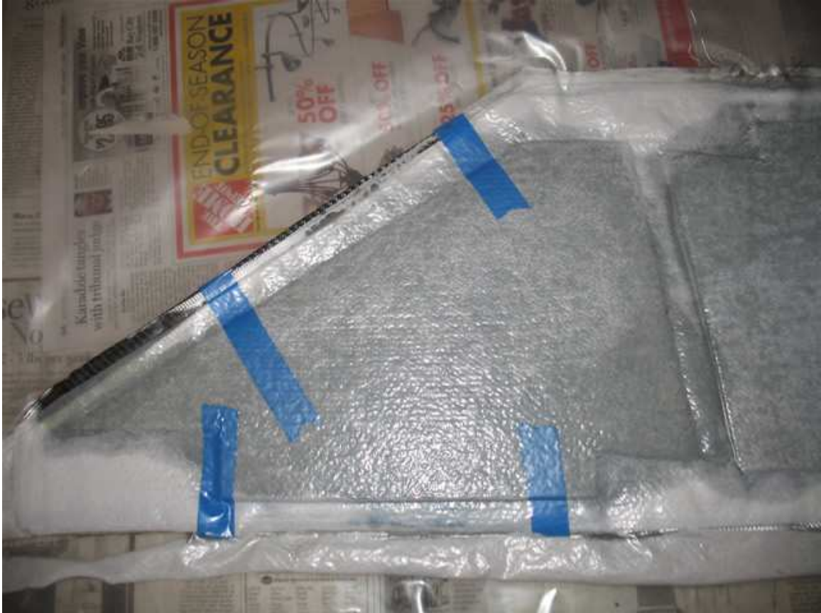
Another view of the layup under vacuum. I get a 24cm vacuum out of my pump, or about 10lb / sq foot I would guess.
