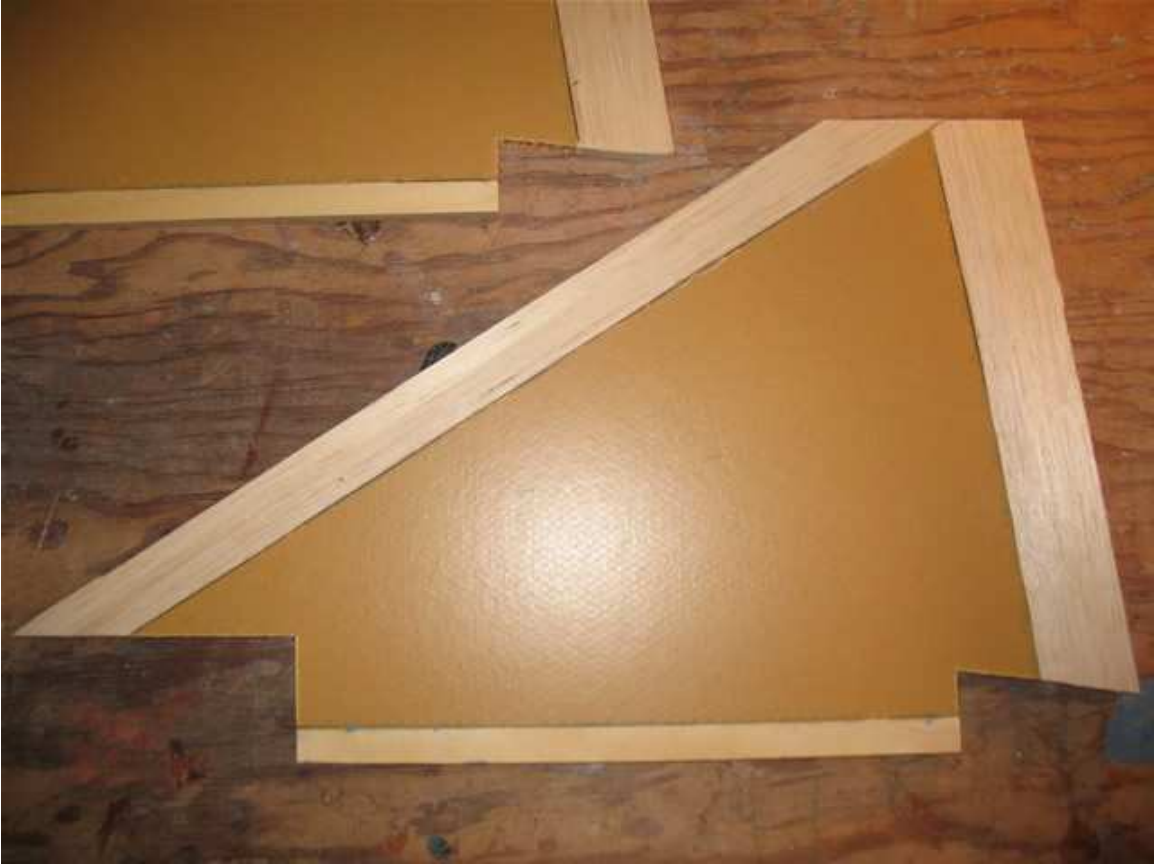
The fin edging is now ready to shape.
