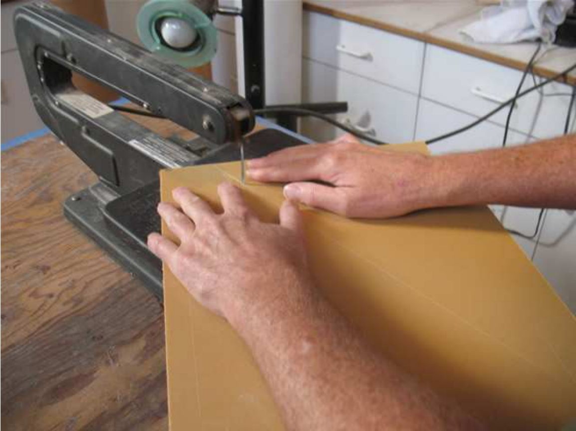
I cut the honeycomb using my old Dremel scroll saw. It cut very easy.
