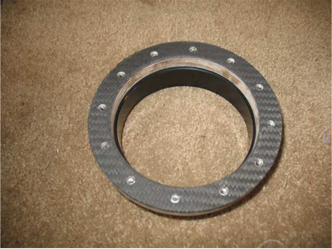
Here is the ring with the Aeropac retainer mounted. Perfect alignment!
