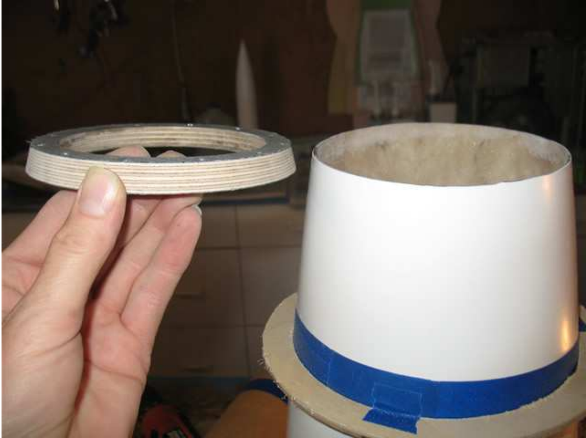
Here is the final ring ready to be epoxied to the motor mount.
