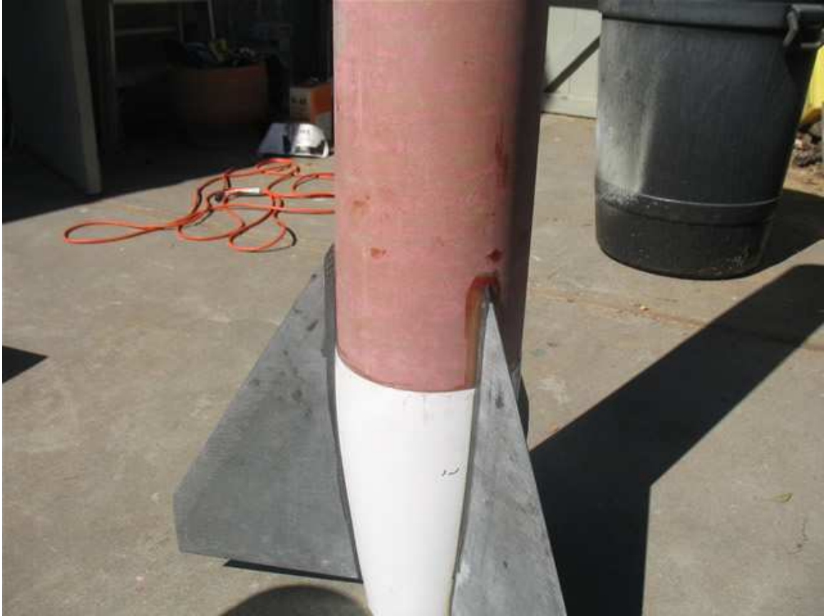
Here is the bottom of rocket assembly hardening in the sun. I added epoxy to the forward edge of the fins to attach these.
