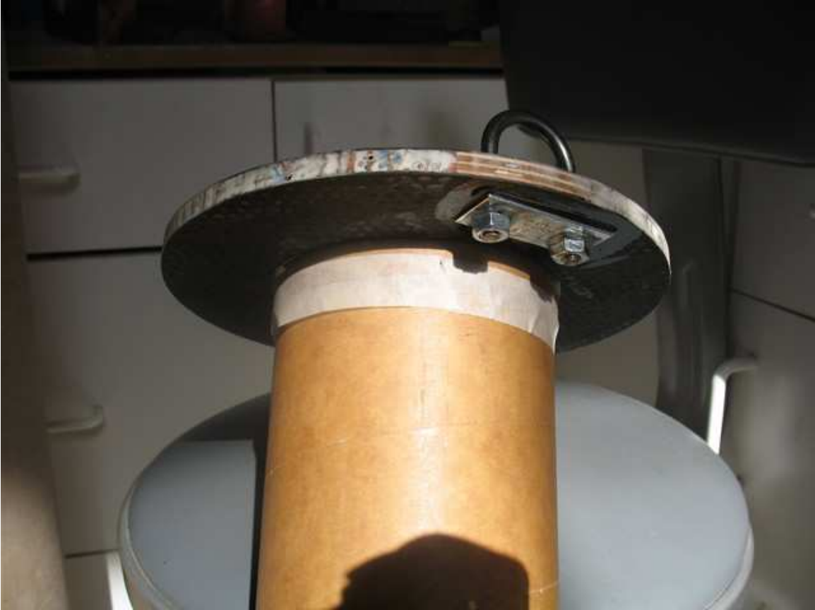
Bottom view showing the U-bolt mounting plate. Note the U-Bolt is mounded onto the inlayed plywood laminated between the carbon reinforcement.
