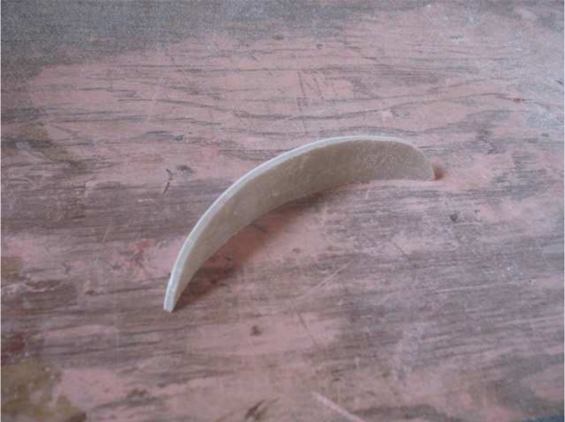
Here is the fiberglass reinforcement shaped from a piece of tail cone shoulder.
