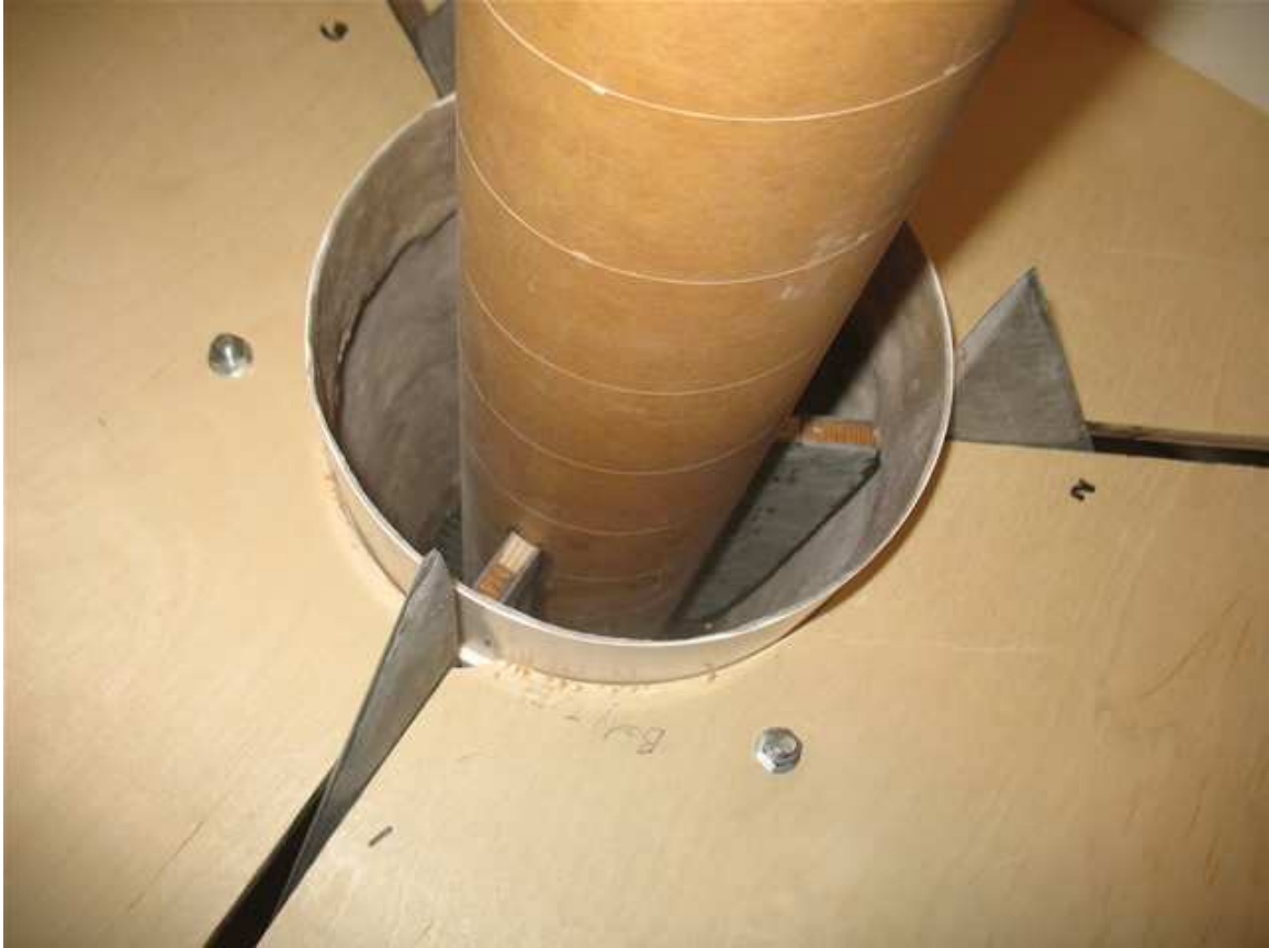
After the first fin is glued the other two are as well using the jig for alignment.
