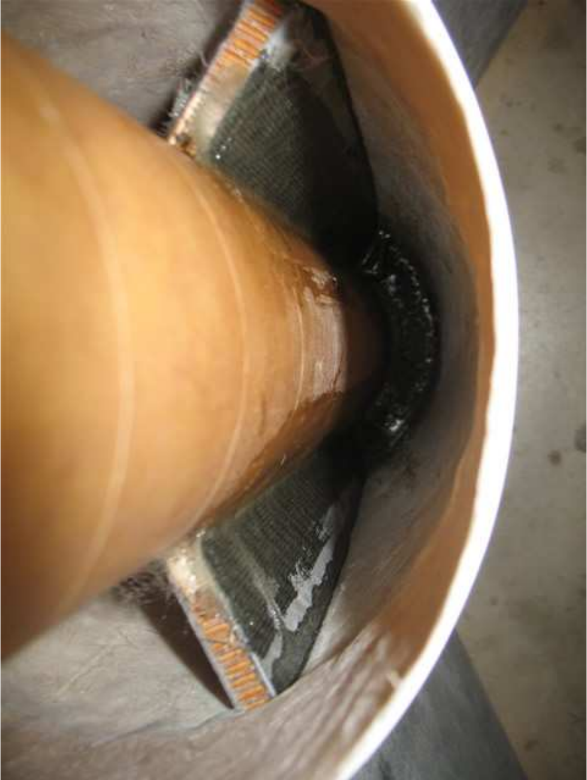
Here you can see the glass reinforcement on the fin tab to motor mount connection. Similar reinforcement is done from the fin tab to the boat tail.
