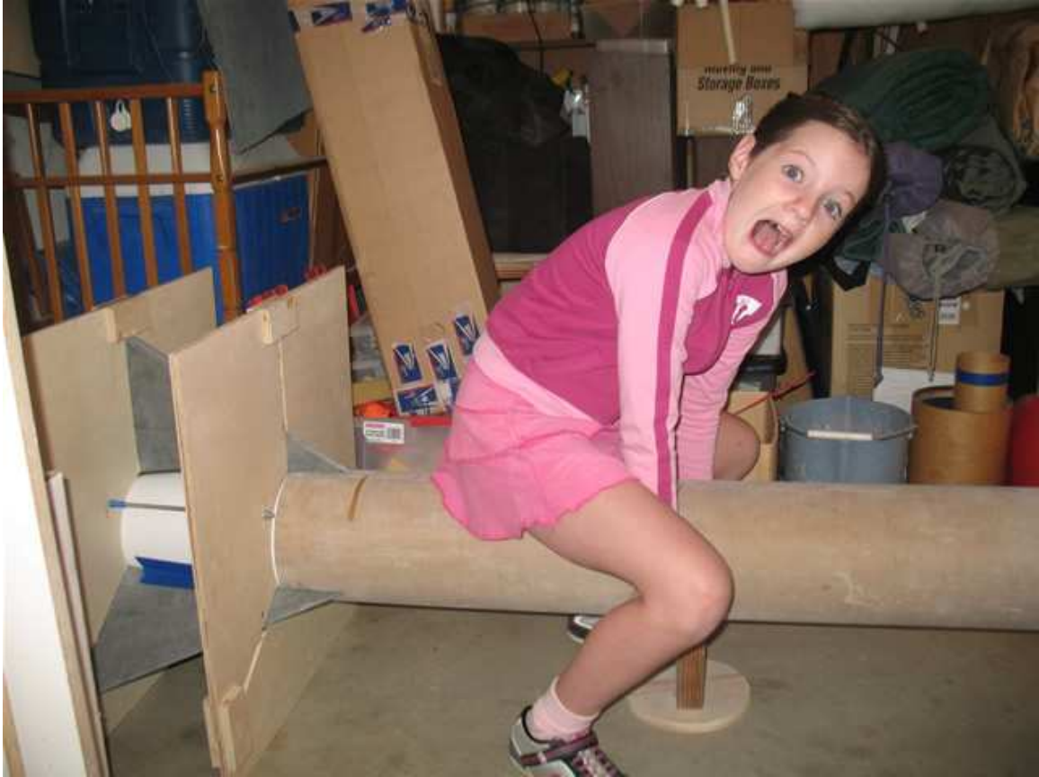
The airframe is also used to help keep the engine mount exactly centered. Jayne thinks she might be able to ride the rocket ala Slim Pickens in Dr Strangelove. But I think Slim sat backwards...
