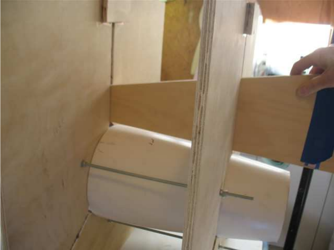
Pieces are ply wood are used to insert into the slots so the slot positions can be exactly marked.
