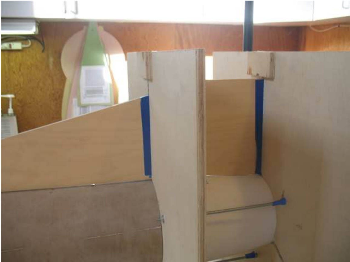
Here is another view. The wood extends up the airframe (not yet attached) and is used to make sure the fins are lined up with the center line of the airframe.
