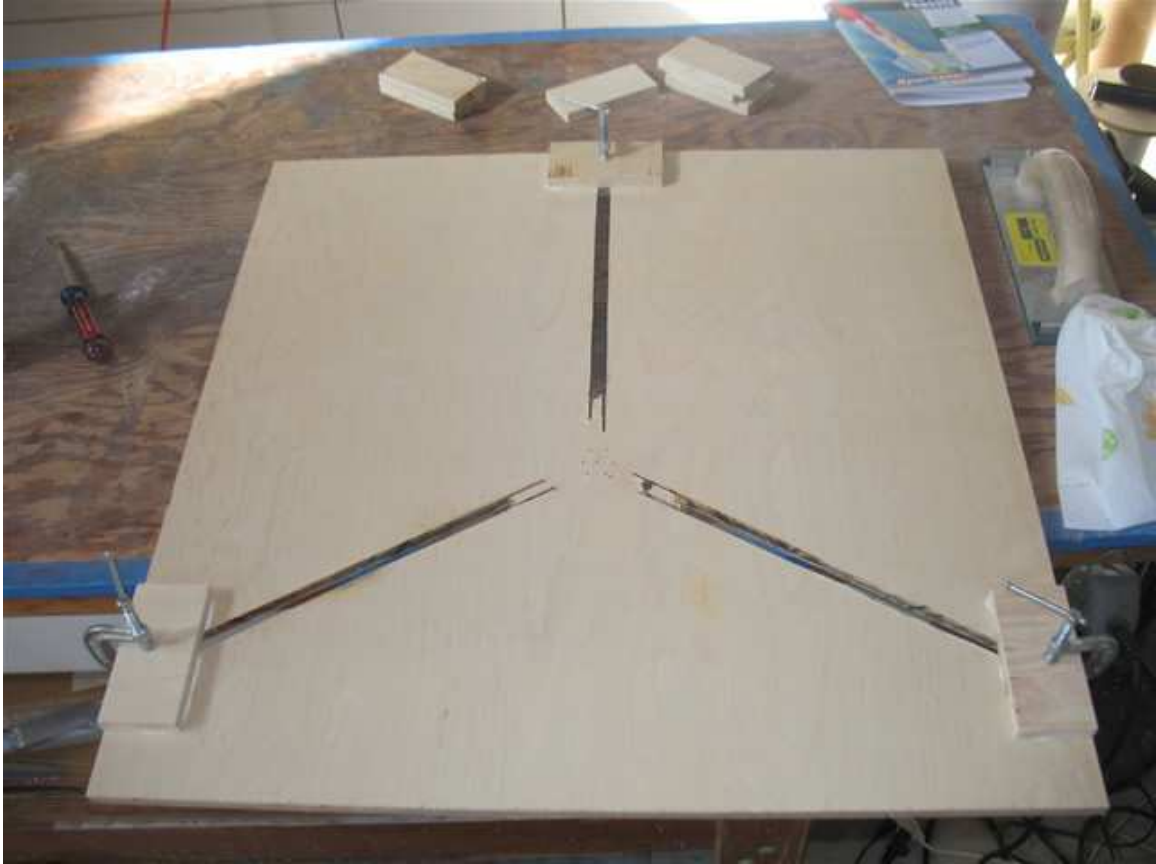
After cutting the pieces are separated. Since the slots approach the edges an extra piece of ply is glued to the tips to stiffen these up.
