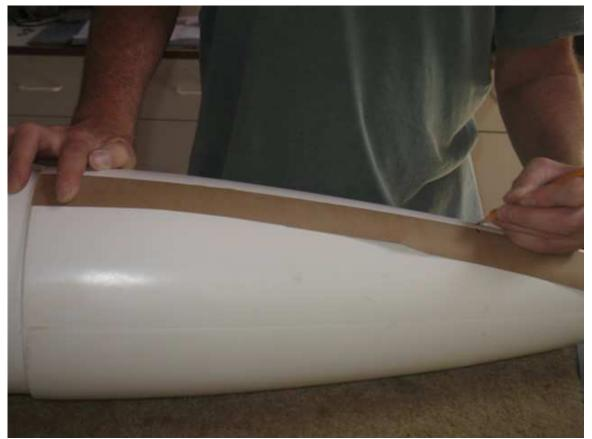
Ok, this is better, I used a paper strip with a mark so when laid on the curved surface it would yield exactly 14" from the shoulder. Using this I made a series of marks around the nosecone every few inches. From past experience it's really hard to eye-ball this sort of cut.
