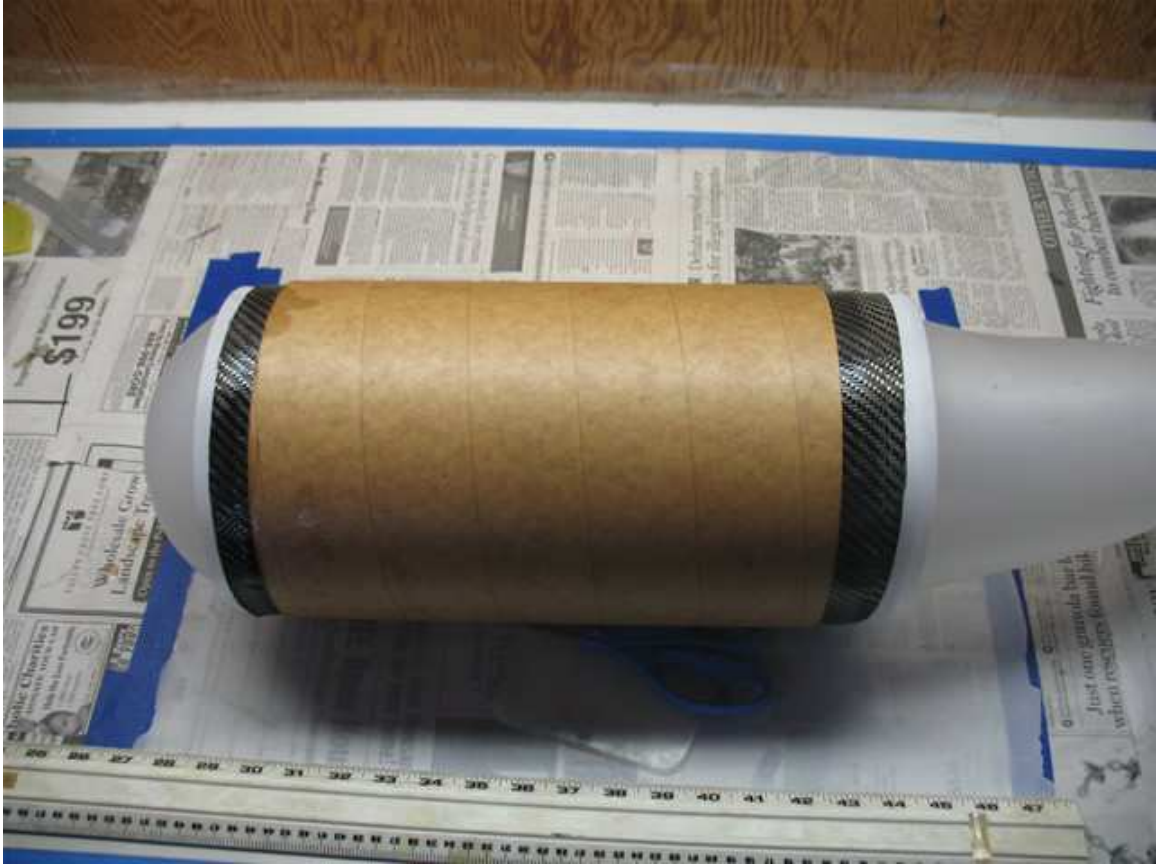
The coupler is lined with two layers of 3K twill. I "balloon bagged" it to make sure I had a tight bond to the coupler inside.
