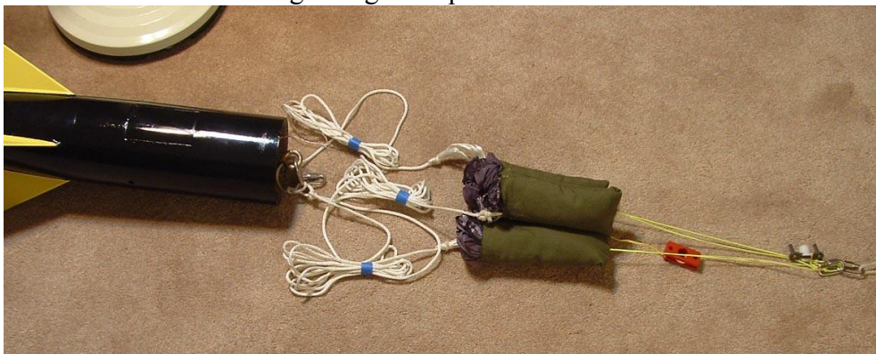
Mains are pulled from the Airframe...
