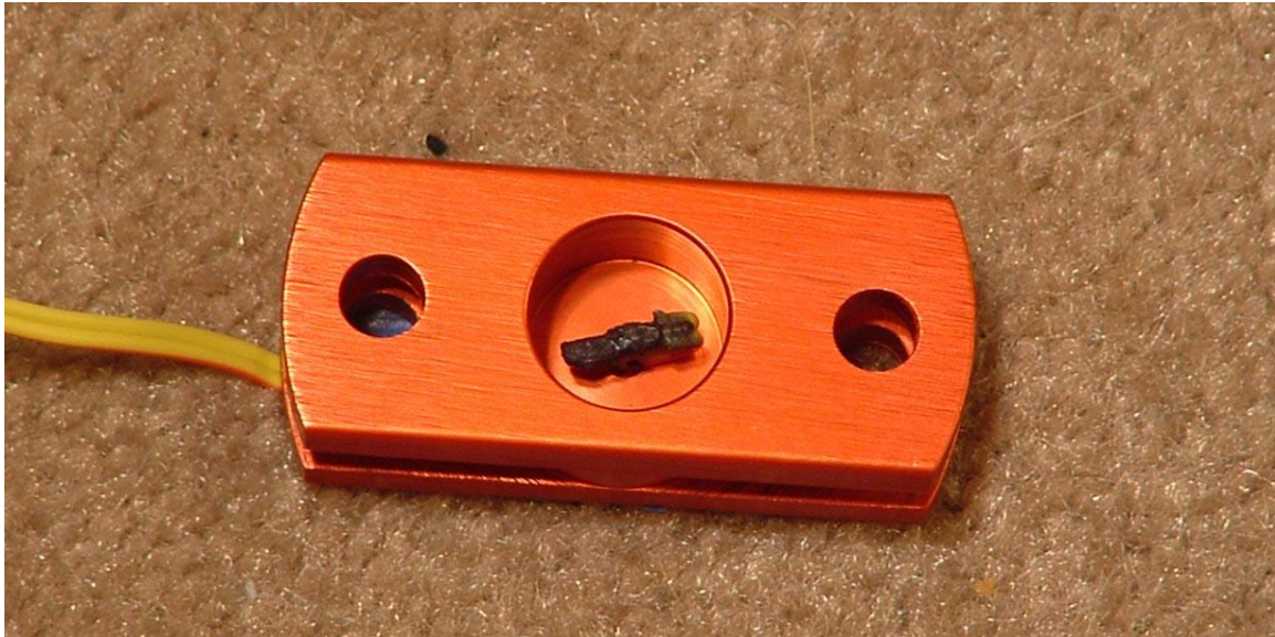
“Davey” type electric match chip – Method 2
