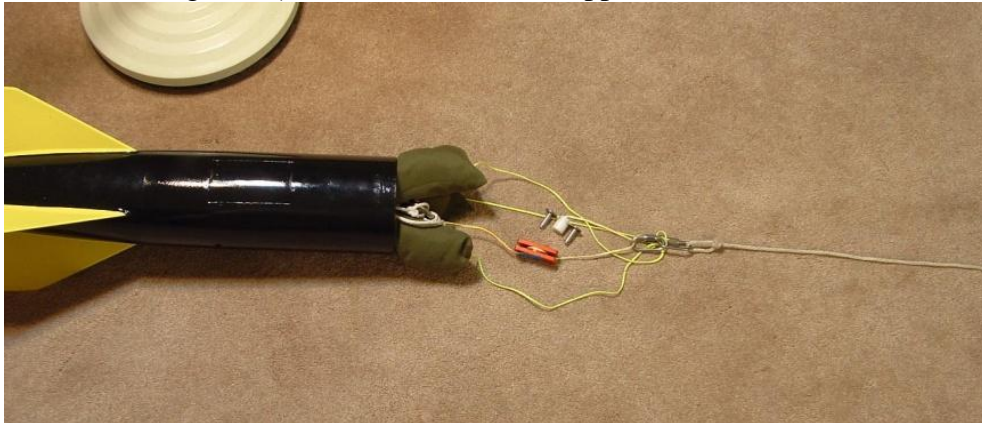
Tender Descender “pops” and releases... (Blue tape on bags is removed for clarity)
