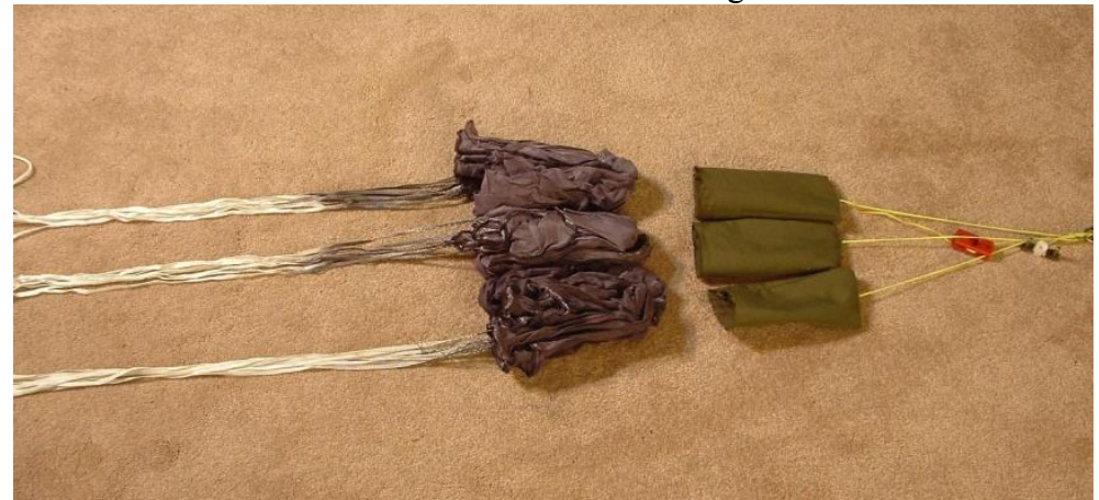
Chutes are out and can deploy with virtually no chance of entanglement! (Note: The Tender Descender goes “up” with the bags and the drogue!
