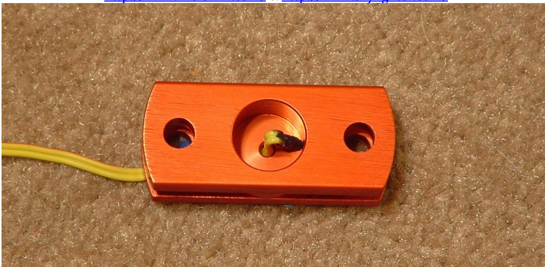
“Davey” type electric match chip – Method 1
