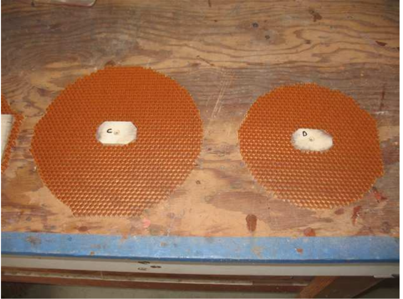
This shows the middle rings that flank the fin tab. Note the right one is smaller to accommodate the boat tail.
