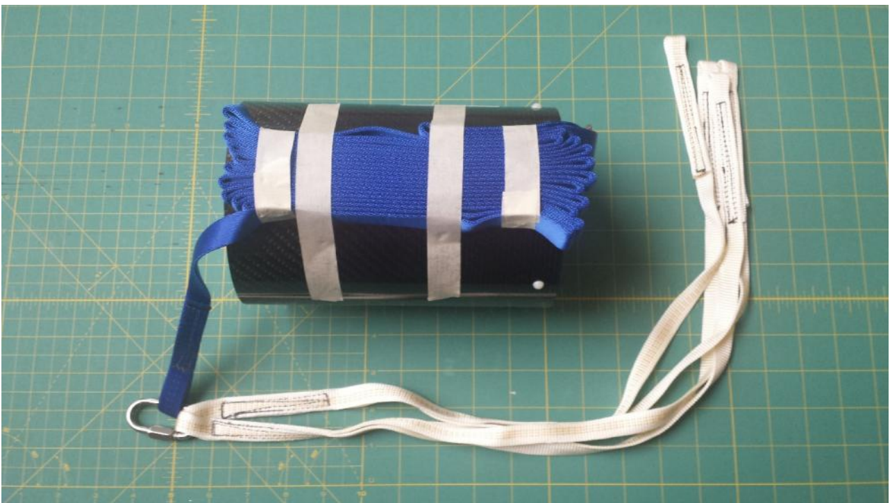
Simple way to attach the main shock cord to the canister for Multi Copters where the speed is lower. Upon parachute deployment the tape is broken easily and the cord extends.
