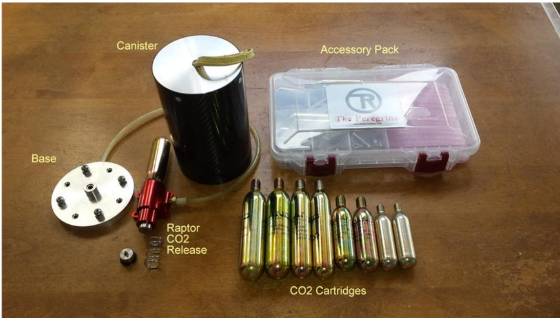
The Peregrine UAV Hardware Kit with the Raptor CO2 Release
