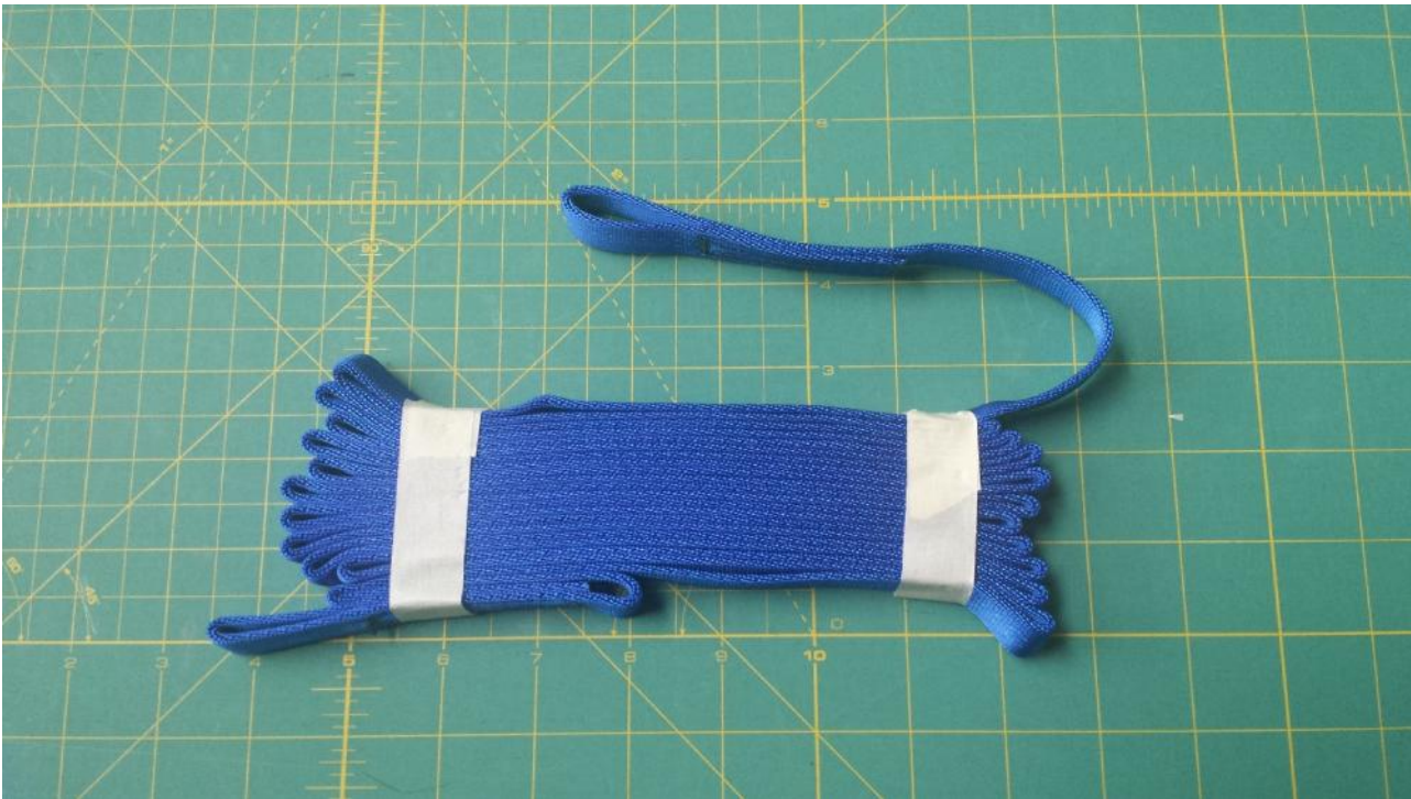
Example of Z-fold and taping of a 5 yard 3000# Shock cord
