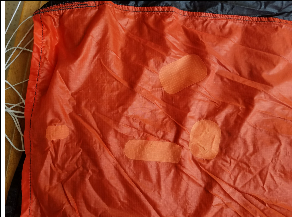
Outside of chute showing finished repair.
